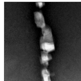
Cr-rich precipitates on a grain boundary in 304 stainless steel
